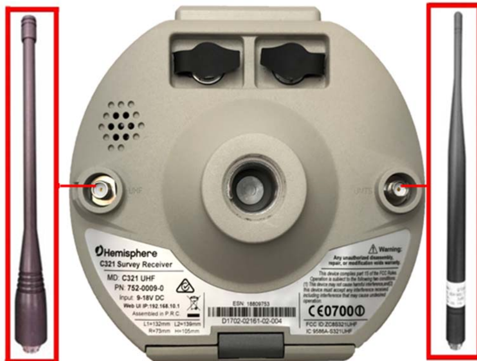
Figure 2-3: Installing UHF and GSM Antennas
